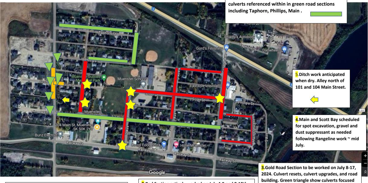
1. Green road Sections complete - July 3, 2024. Shaping, base gravel and top gravel. Yellow Stars show Culverts improved/replaced.
